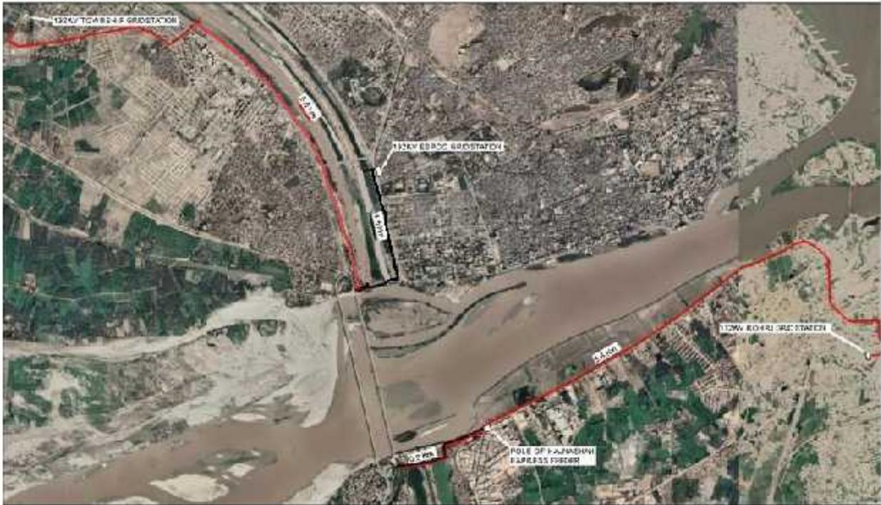
**Figure 2.11: Options for 11 kV power line on right and left banks**
